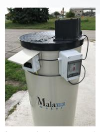
the necessary amount of water in the dosing unit, and mixed in the microbial products, you just need to turn on the main switch, and aeration starts.
