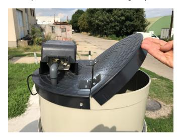
The unit is constructed for suspensions, or solutions, easy to operate, and keep it clean. Activation of microbes is done by coarse bubble aeration. Air is supplied by a small capacity blower placed at the top the machine. Whenever you put
