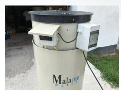
or solution can contain solid residuals from the manufacturing process. That can easily lead to continuous clogging of metering pumps. We have created Malatech-C Dosing Unit for reliable, and trouble-free continuous dosage of biotechnological products.
