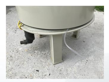
Considering the nature of biotechnological products, we recommend to open the bottom valve before every refill, and clean the unit by flushing the inside part with pure water.
